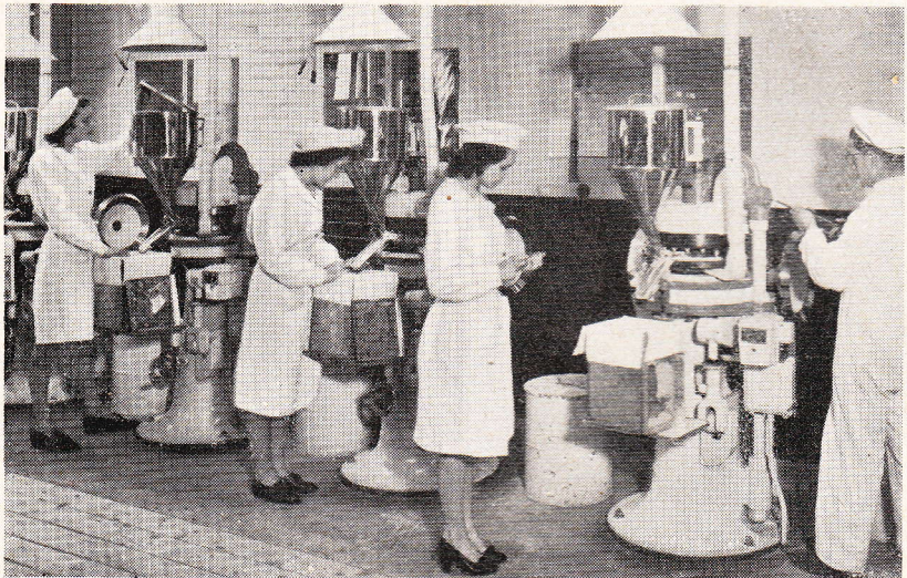
These machines compress the Tibs Worm Tablets for cats. Each machine is capable of producing 320 tablets a minute.
