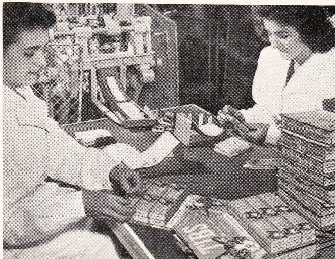
Loading cartons with Tibs Cat Powders. One of the powder wrapping machines is shown in the background.
